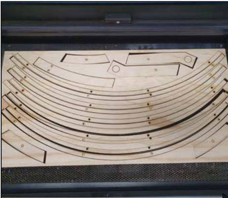
The parts were laser cut in stages and parts placed with the same types. This ensures the right number of pieces is printed.
