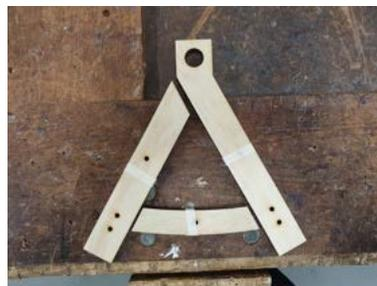
After more parts were cut out the structure of the frame started coming together. However, the realisation was made that the original intended laminating thickness was going to be too thick. The original design noted 14 layers of plywood or 42mm in thickness. The sheer weight of this many lamination
