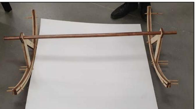
This is the last assembly before fixing all the components together. This is also the first time the frames have interacted with both the corflute and copper pipe. It was found in this assembly test that the frame may not have enough integrity to hold the corflute steadily in place.
