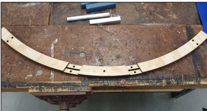
Both sections of the frame was now glued on after waiting for the rear curved part to 'de-warp'. At this point the process will be repeated for the 2nd frame.
