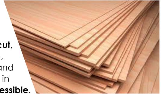
**Disadvantages:** Plywood, although quite enduring, is **not the most durable** wood, compared to other solid woods. It does tend to **chip** quite easily and when compared to other woods, does **not handle wet weather or moisture very well**. Also, if plywood is sanded to the extent in which the top layer is removed, the surface of the wood will display an unappealing surface.
