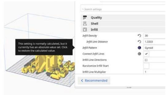
For the fingers and palm prints, I had to create support blockers for all of the smaller holes and structures in the model, to prevent structures from being built in there, as these are almost impossible to remove.
