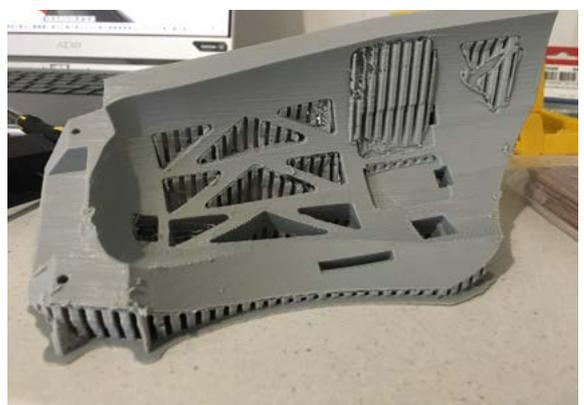
For the smaller support holes, I was able to use a combination of pliers, a stanley knife and scissors to scrape off the remainder of the support materials which stubbornly remained on the surface of the prints.
