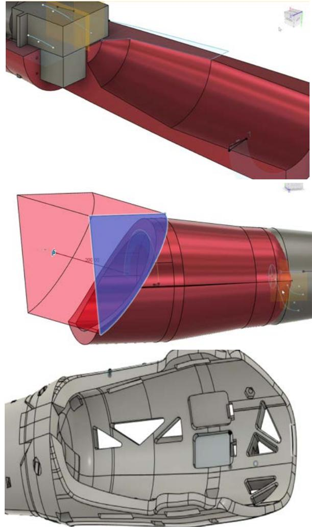
1. For the Electronics casings I did a quick outline of the minimum boundaries required to contain the electronics.
