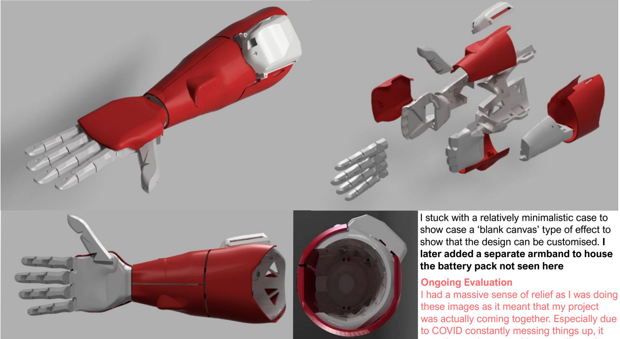
I stuck with a relatively minimalistic case to show case a 'blank canvas' type of effect to show that the design can be customised. I **later added a separate armband to house the battery pack not seen here**
