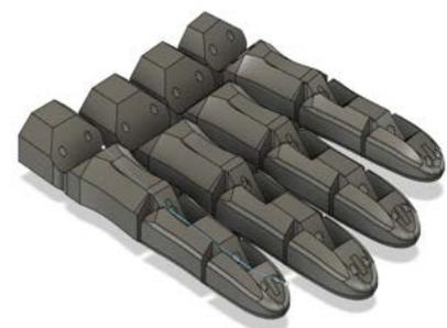
4. I then sculpted the outline of the fingers with curves and used the fillet tool to curve the corners of the rectangles, being careful that these changes do not interfere too much with the existing structures. This stage included a lot of trial and error to get an aesthetic model that resembled fingers.
