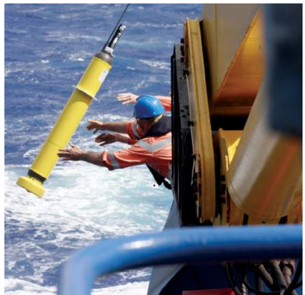
Deploying a robotic Argo ocean profiling float – Alicia Navidad, CSIRO
