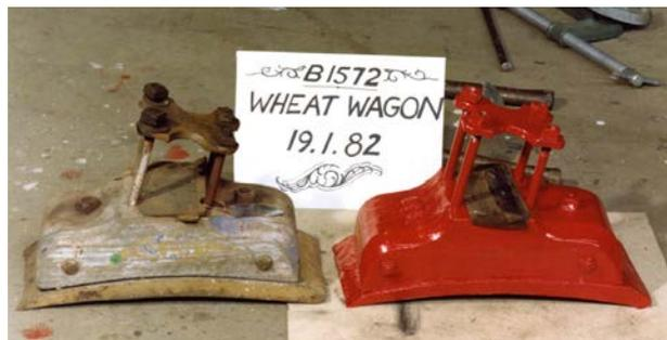
Brake pads showing the original condition and the restored condition.
